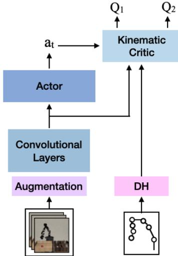
Fig. 2: Kinematic Critic Architecture: differentiate through the Denavit-Hartenberg Kinematics during training. Note that the sampling of action  $a_t$  admits differentiation with respect to the action distribution predicted by the actor, using the reparameterization trick [9], [10].
